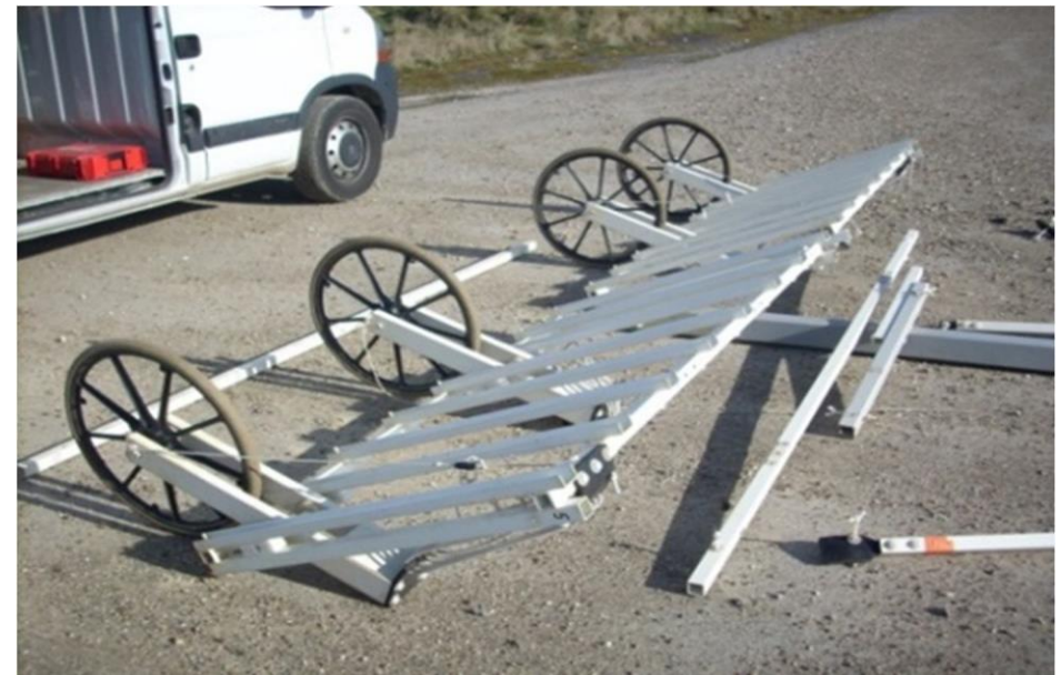
Example of mounting an 8 probes frame
