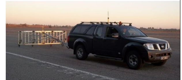
Example of different types of fluxgate devices: 4 VALLON georeferenced sensors (top left), Foerster monoprobe (top right), 8 EBINGER/SENSYS georeferenced sensors towed by a vehicle (bottom)
